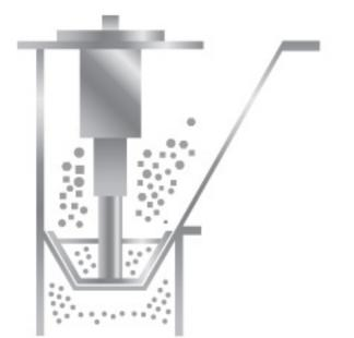
Unprocessed material is **UmacMill** into the product **imyethantich**, gravity feed or <u>vacuum transfer</u>. The material The material is instantly reduced in size as it passes through the holes in the screen.
