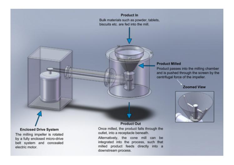
Material is fed into the cone mill via the in-feed chute, using hand-feed, gravity-feed or vacuum-feed. The material passes into the milling chamber, where the centrifugal force of the rotating impeller pushes material through the apertures of the screen (this process ensures that material will not pass through the screen until the particle is the desired size).
