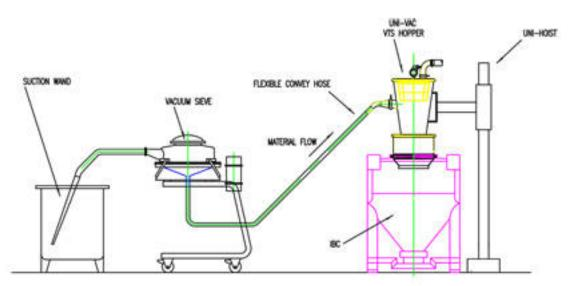
Using vacuum transfer, processes such as milling and sieving can be performed 'in-line'
